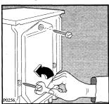
Remove the polystyrene base, set the machine upright and unscrew the two remaining rear bolts.
